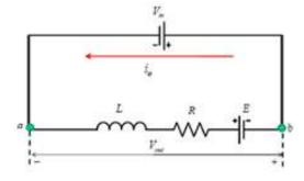
Fig.7 (a) Reverse Motoring
