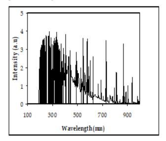
Fig 3: Spectrum of UV lamp radiation
