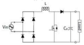
Fig 2. Fundamental design of boost PF correction circuit
