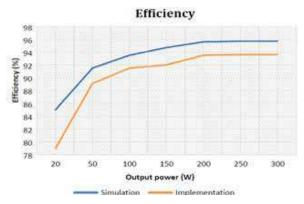
Fig. 10- The proposed DC-DC converter's efficiency
