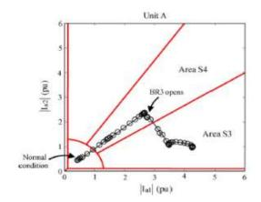
Fig. 8 Trajectory of the current amplitude of phase A for 6th case of table 5
