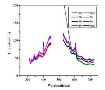
Fig. 4 (c) PL characteristic of BaB<sub>8</sub>O<sub>13</sub>: Sm<sup>3+</sup>
