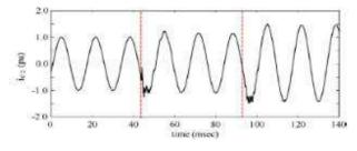
Fig. 3 Current waveforms at L\_G fault of ckt. 2
