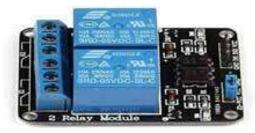
Figure 4: Relay module
