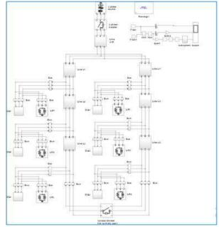
Fig. 16: Microgrid islanded mode of operation
