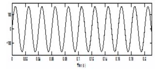
Figure 13: output produced by inverter after filtering (Phase a)
