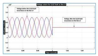
Fig. 14: Voltage nature for LLLG fault on line L1 before and after the fault
