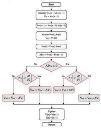
Figure 3: Flowchart for the P & O MPPT algorithm [1]
