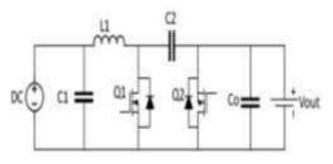
Fig.6.b Bi-directional dc-dc Cuk converter
