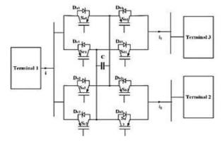
Fig.6. H-Bridge Dual CFC Topology
