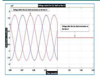
Figure 9: Voltage nature for LLL fault on line L1 before and after the fault occurrence
