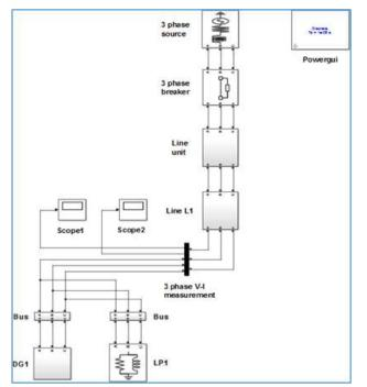
Fig 12: Microgrid system with one DG connection for LLLG fault on line L1
