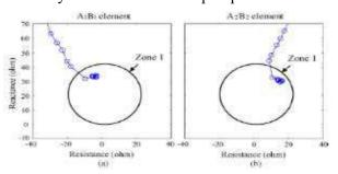
Fig. 11 Measured impedances by A-B elements of the conventional distance relay for the inter-circuit A1B2G fault on the transmission line (a) Impedance of circuit 1 (b)
