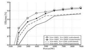
Fig. 11 Efficiency curve of the three-level converter
