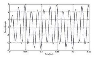
Figure 10: Current waveform excluding PSO
