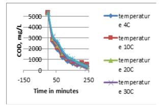
Fig 7: Effect of temperature on COD removal rate of detergent. pH = 5.5, catalyst concentration 125 mg/L, detergent concentration 1250 mg/L
