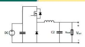
Fig.5.a Unidirectional Dc-Dc Buck System
