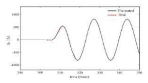
Fig. 10 estimated zero-sequence current of circuit 2 for the external fault on the transmission line BC.
