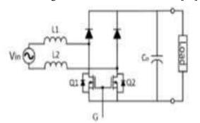
Fig. 3. Fundamental design of conventional boost PF correction.
