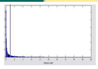
Figure 15: Waveform investigation of output current using FFT
