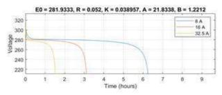
Fig. 2 discharge characteristics at different loading
