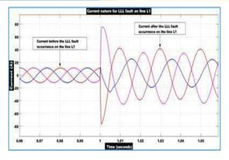
Figure 10: Current nature of LLL fault on line L1 before and after the fault occurrence
