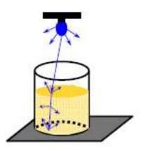
Figure 1: Simple slurry phase photo-catalytic reactor
