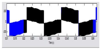
Figure 12: Phase-to-phase output of a 3-Ø inverter
