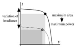
Figure 2: The Solar Cell's I-V Phenomenon
