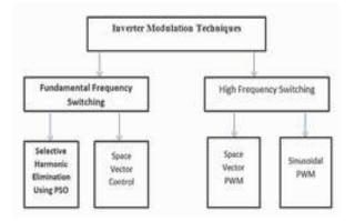
**Figure 1. Strategies for Modulating Inverter Outputs**
