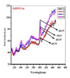
Fig. 4 (a) PL characteristic of BaB<sub>8</sub>O<sub>13</sub>: Sm<sup>3+</sup> excitation
