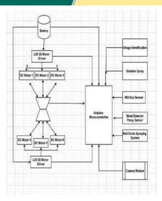
Fig. 1- Block diagram of Six-leg pipe inspection robot
