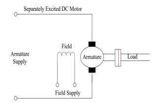
Fig 9. DC separately excited motor
