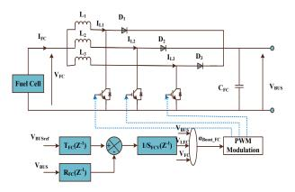
Fig.5.Control of VDC bus
