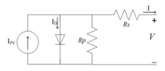
Figure 2: Solar PV single diode circuit
