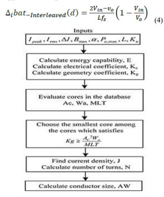
Fig. 7. Flow diagram for the core geometry estimation approach-based inductor design method
