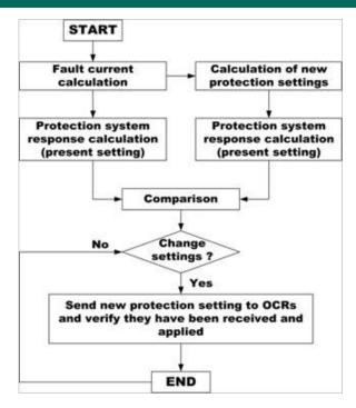
Fig. 2: Adaptive overcurrent protection algorithm
