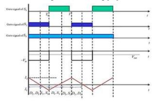
Fig.8 Output Waveform of third and fourth quadrant
