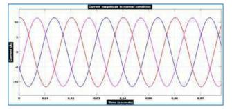
Figure 6: Current magnitude in normal operating condition
