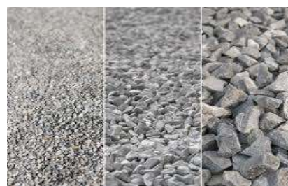
Figure 2: Aggregate fine, 10 mm and 20 mm.
