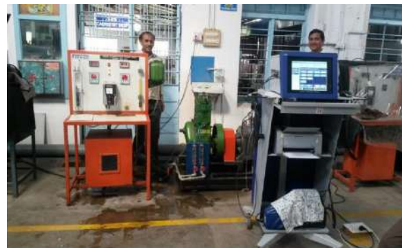
Figure: 3.1 Diesel Engine Test Rig with AVL DiTEST (Exhaust gas analyzer)
