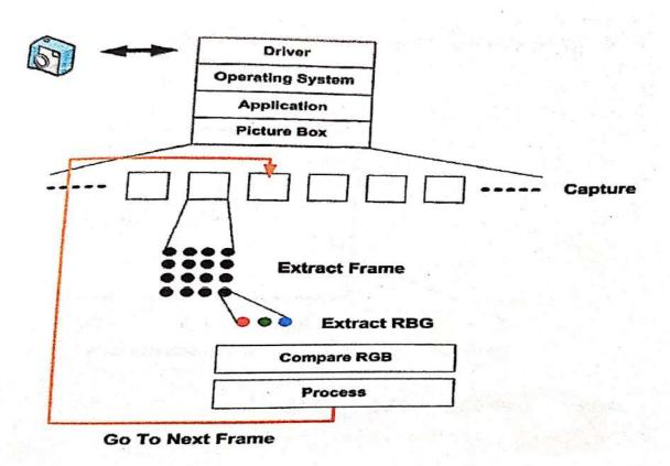
Fig. 4: Image processing algorithm flow
