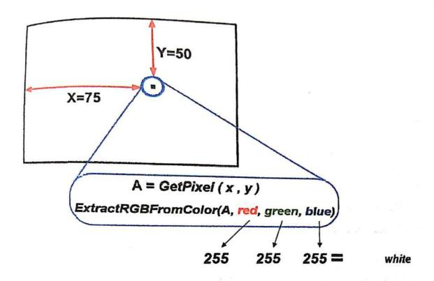
Fig. 5: Pixel colour extraction method
